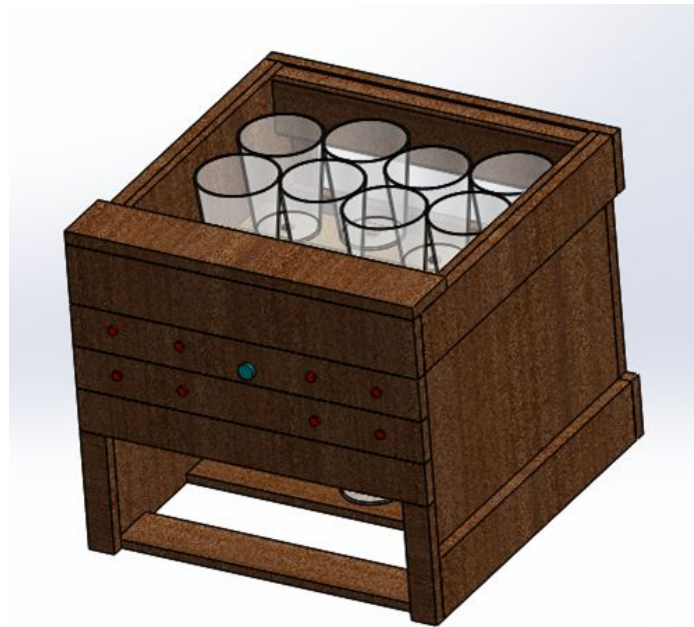
Figure 4A: The final CAD product, storing 8-1 L containers, and our user interface.
